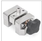
\* Reverse the jaws to switch from ØD1 to ØD2 Includes a #10-32 M/M stud with jam nuts
