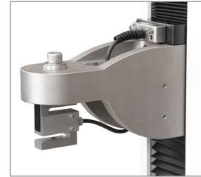
Install the sensor to the underside of the crosshead using the supplied socket head screw and hardware. Plug the connector into the connector into the receptacle in the top front surface of the crosshead, then fasten the two thumbscrews, as shown at left. Grips and fixtures may be threaded onto the underside of the sensor.
