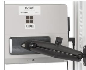
Test frame part numbers ending in "-IMT", for example Model F1505-IMT, include a Windows tablet with attached ball mount and mounting bracket, packaged separately. The mounting arm is pre-installed into the front right slot in the test frame column via two screws.
