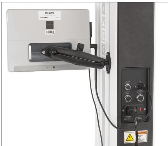
Plug in the AC adapter and press the Power button, in the lower right corner of the tablet. The tablet will boot up directly into the IntelliMESUR application. If not, select the IntelliMESUR icon in the Windows home screen.
