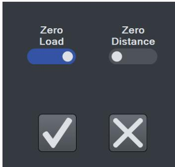
A **Zero** step zeroes the load and/or distance. Make the desired selections.
