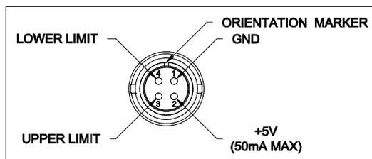
Note that when pins 3 and 4 are not connected, the auxiliary limits are inactive. When the +5V from pin 2 is connected to either pin 3 or pin 4, the respective limit becomes active and the crosshead is prevented from movement in that direction.
