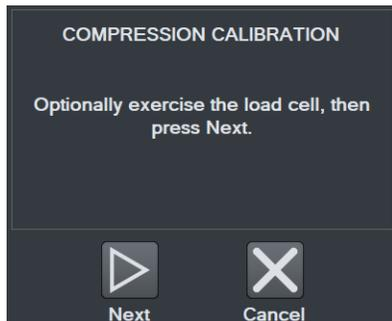
Optionally load and unload the force sensor to full scale several times, then select **Next**.
