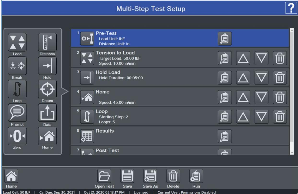
The step sequence must contain the three steps listed above: **Pre-Test**, **Results**, and **Post-Test**. To edit these steps, select **Edit**, and configure the parameters the same way as in **Basic Test** setup.
