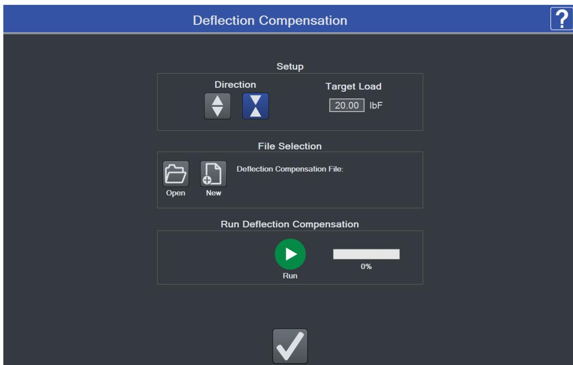
3. Configure the direction, tension or compression, then set the target load.
