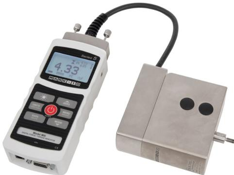
The optional extension cable part no. AC1084 can be useful in addition to AC1083 where the indicator cannot be positioned close to the force sensor.
