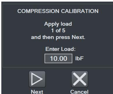
Apply the indicated compression load using the **crosshead motion controls**. The load value defaults to even intervals. For example, for a 50 lbF force sensor with 5 calibration points, the first default load value is 10 lbF. All load values may be edited by up to  $\pm 20\%$ .
