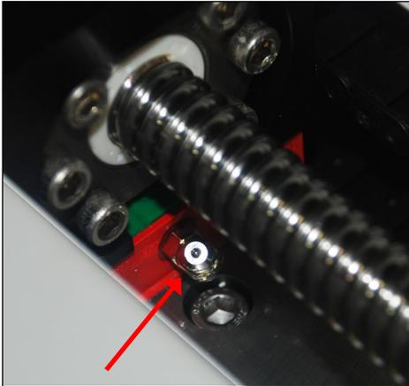
4. Using a grease gun, add general purpose bearing grease to the inside of the slider until full. Wipe clean any spillage. Refer to the image below:
