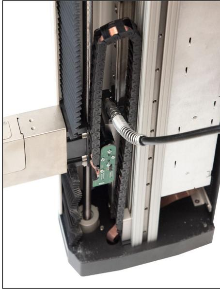
7. Cycle the crosshead up and down several times until the newly applied grease has been spread evenly over the length of the slide.
