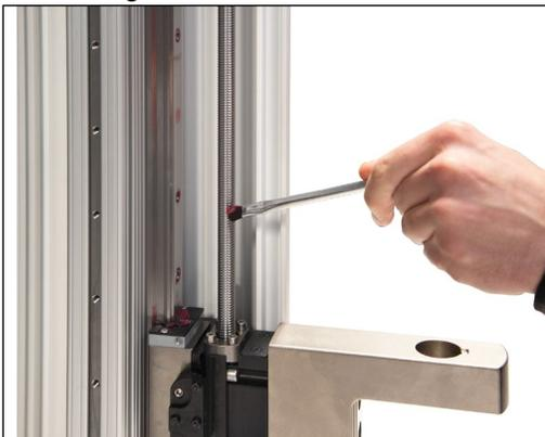
3. Cycle the crosshead up and down several times until the newly applied grease has been spread evenly over the length of the screw.
