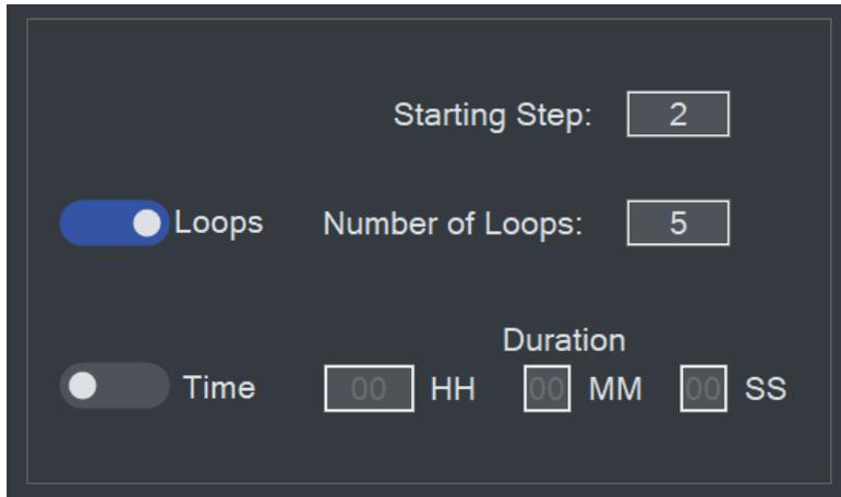
The **Loop** function repeats a range of steps. Insert this step after the last step to be repeated.
