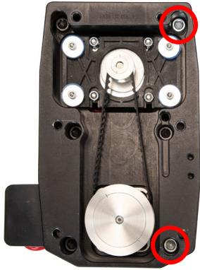
4. Remove the Mark-10 logo strip, then remove all screws from the side of the test frame, as shown below:
