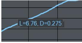
The cursor will snap to the closest plot when multiple runs are displayed simultaneously.
