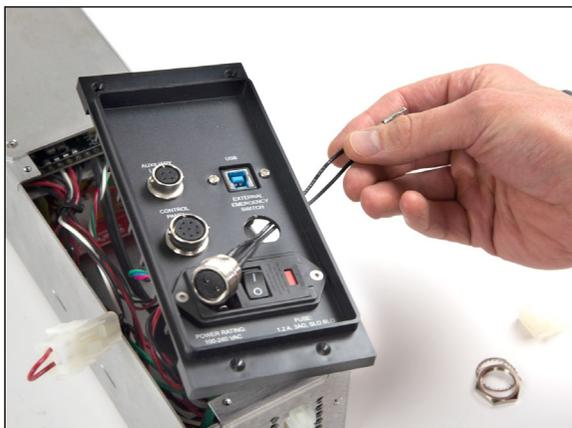
5. Connect the two cables to the white mating plug, as shown below:
