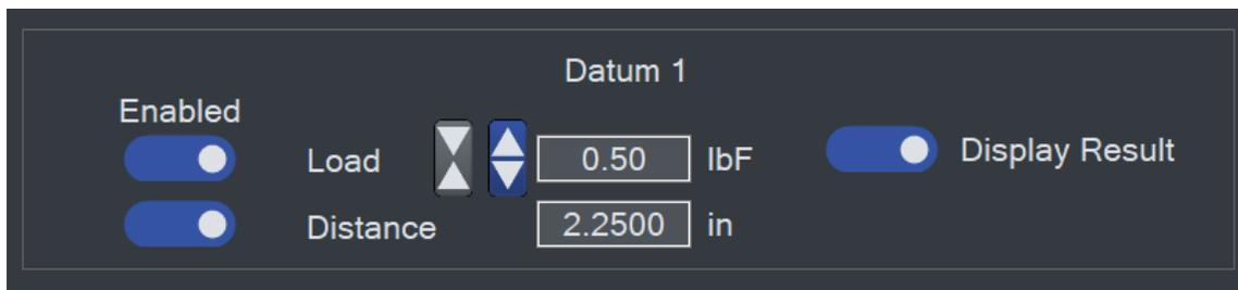
A datum establishes a local offset of load and/or distance. When the datum step is reached, the load and/or distance will change by the values set in the **Load** and **Distance** fields. Enable one or both of these fields.
