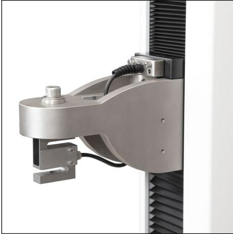
Grips and fixtures may be threaded onto the underside of the sensor.
