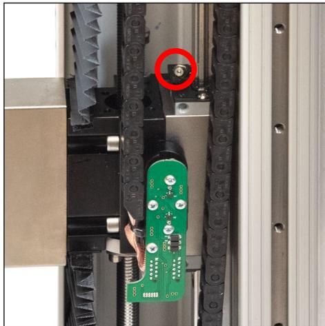
6. Using a grease gun, add general purpose bearing grease to the inside of the slider until full. Wipe clean any spillage. Refer to the image below:
