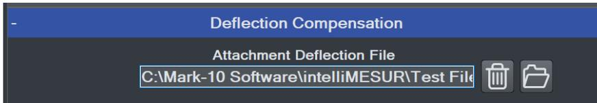
Force sensors and test frames deflect under load, affecting the accuracy of distance measurements. Series F test frames and force sensors are compensated at the factory.
