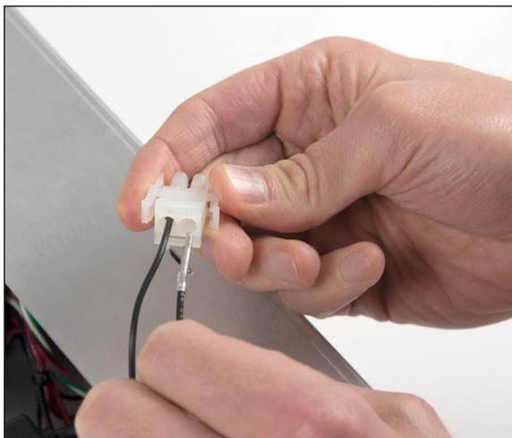
6. Install the connector to the housing by inserting the spacer over the body of the connector, then tightening the nut, as shown below:
