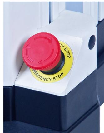
Press down to stop crosshead motion. Rotate clockwise to release the switch.
