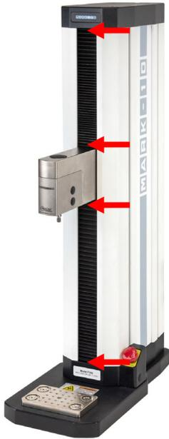
2. Using a brush, apply a small amount of general-purpose bearing grease to the screw, as shown in the image below:
