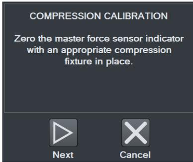
Zero the indicator associated with the master load cell. Engage the calibration fixtures, and ensure that there is no load applied to the force sensor. Then select **Next**.
