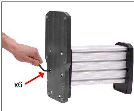
3. Attach the top flange to the bottom of the test frame column utilizing the 6 supplied screws, as shown in the image below:
