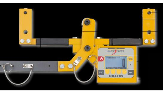
Sheaves with bearings eliminate friction and provide the best accuracy
