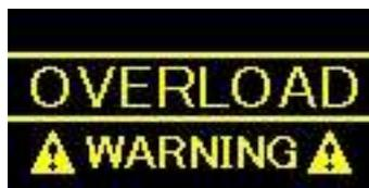
When load over its capacity is added, warning is indicated. Please stops measurement immediately when this indication show up.
