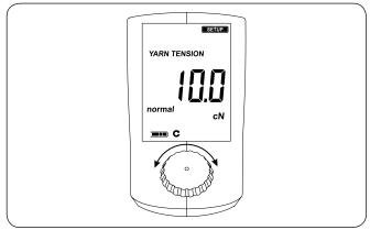
► If the MLT WESCO does not show 10.0 cN the value has to be corrected by turning the rotary knob.
