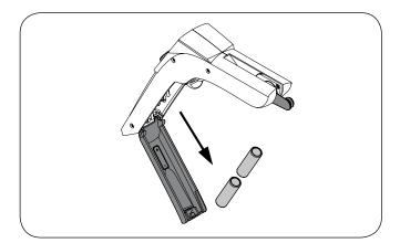
▶ The batteries can now be removed and replaced.
