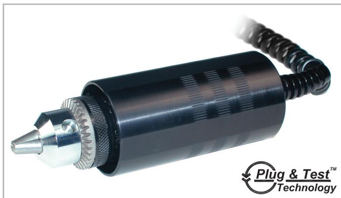
Series R50 smart sensors measure bi-directional torque for a wide variety of applications across virtually all industries. Contain a Jacobs chuck for up to 0.5 in [12.7 mm] diameter samples, bits, or fixtures. The sensors can be used as hand held devices, or mounted to a test stand. Capacities available from 10 ozFin to 100 lbFin [7 to 1150 Ncm]. Compatible with Mark-10 indicators (sold separately) through unique Plug & Test™ technology.
