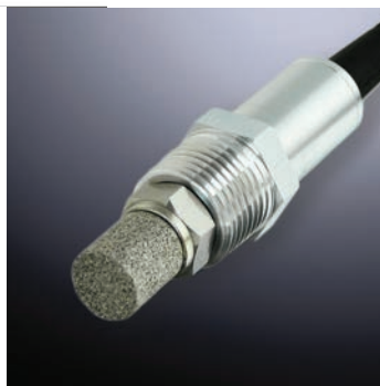
PosiTector DPM D probe includes 1/2" NPT threads for insertion into pipes.
